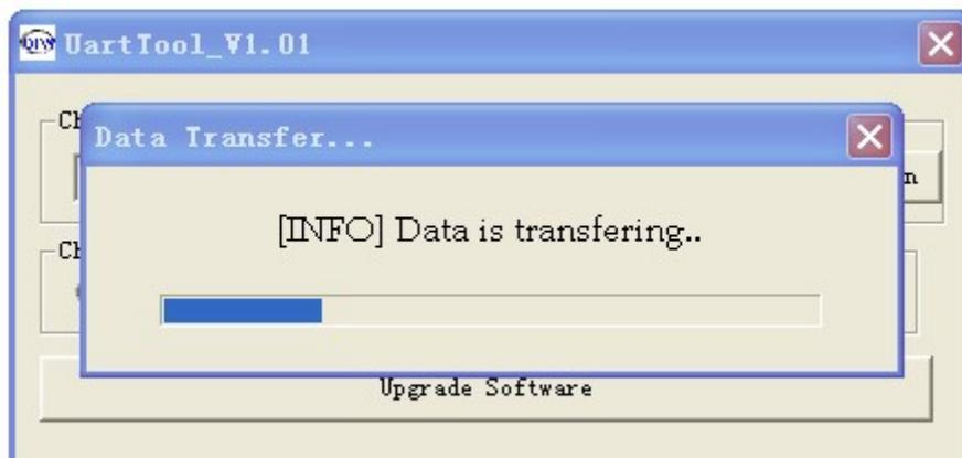
3. About 2 minutes later, the finder will restart automatically, then please go to the “system setting “ submenu, do the “Factory reset”, then upgrading software is successful
